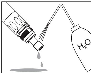
Rinse the sensor head with deionized water.
