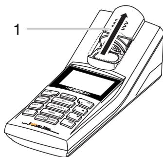
**Inserting a 28 mm cell**
