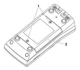
Place four rechargeable batteries (type Mignon AA) in the battery compartment.
