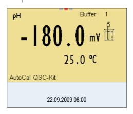
Calibration with the buffers of the QSC-Kit is done like a normal three-point calibration.
