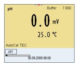
10 Wait for the measurement with stability control to be completed or terminate the stability control and take over the calibration value with < MENU/ENTER>.
