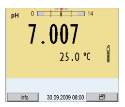
2 Open the *Storage & config* menu with **<MENU/ENTER\_\_>**. The instrument is in the setting mode.
