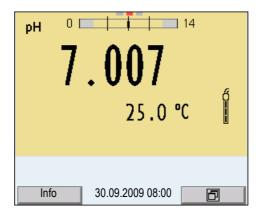
In the measured value display:Display the sensor data (sensor name, series number) with [*Info*].
