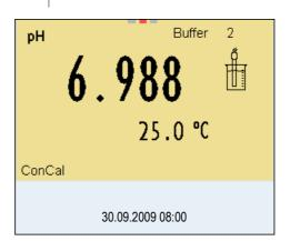
8 If necessary, finish the calibration procedure as a single-point calibration with **<M>**.
