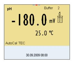
If necessary, finish the calibration procedure as a single-point calibration with **<M>**.
