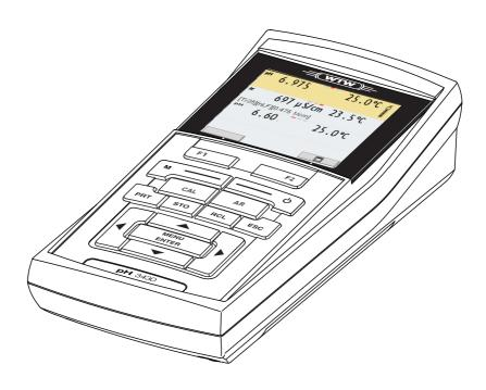
Digital pH / dissolved oxygen / conductivity meter for 3 digital IDS sensors
