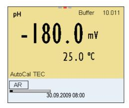
Wait for the end of the measurement with stability control or accept the calibration value with **<MENU/ENTER>**.
