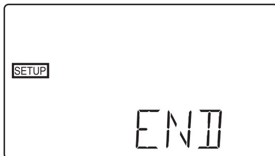
38 Terminate the setup program with
