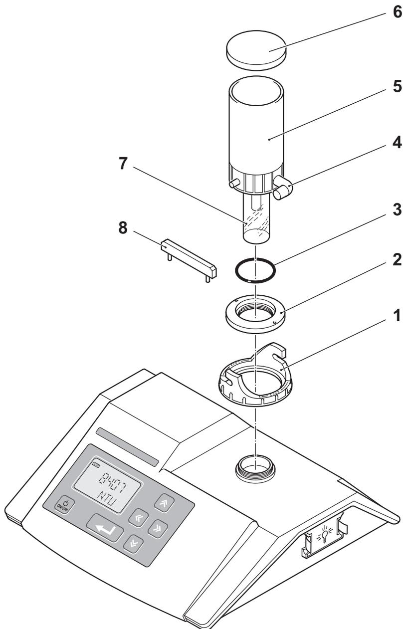
To install the pour-through vessel, proceed as follows:
