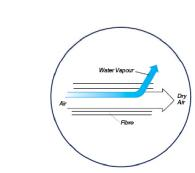
Water vapour quickly permeates the membrane and is released harmlessly to atmosphere. Air flows along the membrane fibre as a separate product stream.
