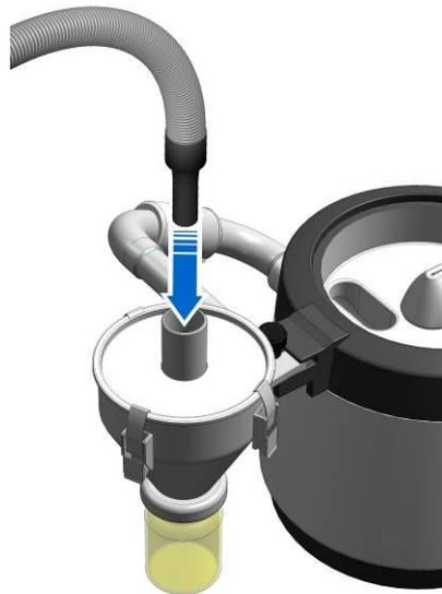
Fig. 19: Connect the vacuum cleaner
