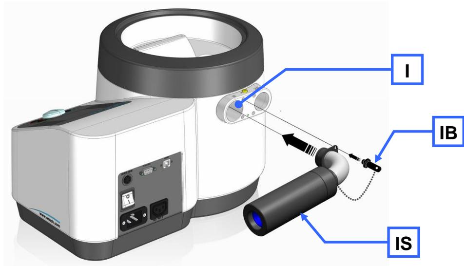
Fig. 1: Connecting the sound absorber
