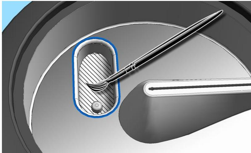
Fig. 21: Cleaning the air outlet channel
