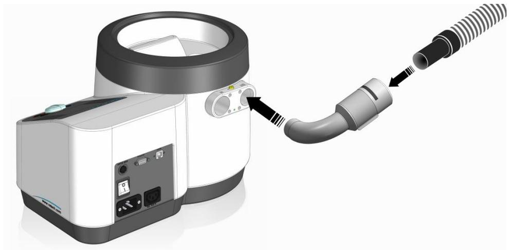
Fig. 13: connecting the manual suction force adjuster
