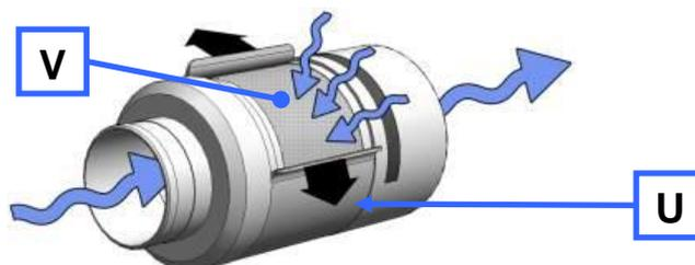
Fig. 11: Air jets through the manual suction force adjuster
