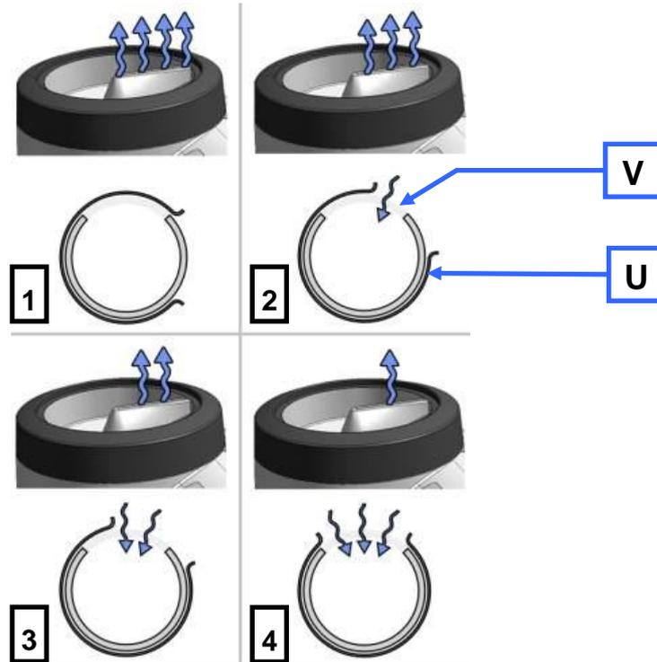
Fig. 12: Manual adjustment of the air jet (cross section)
