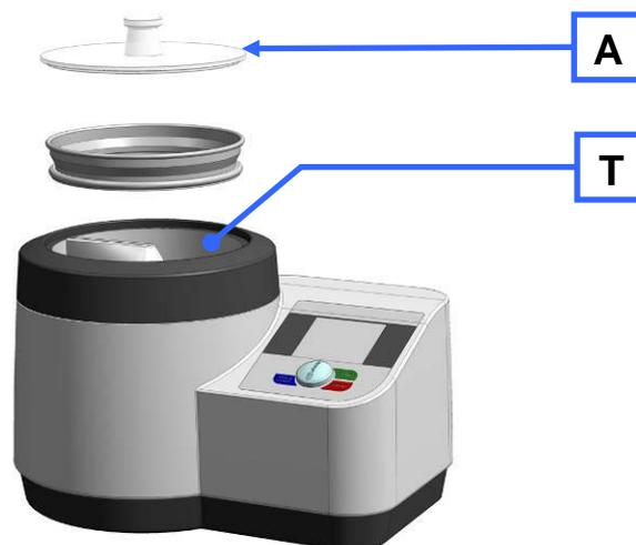
Fig. 7: Inserting the test sieve
