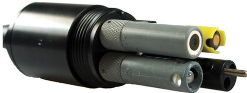
The 10102030 4-port cable bulkhead shown with four user-replaceable sensors including temperature/conductivity, DO, pH, and ammonium.
