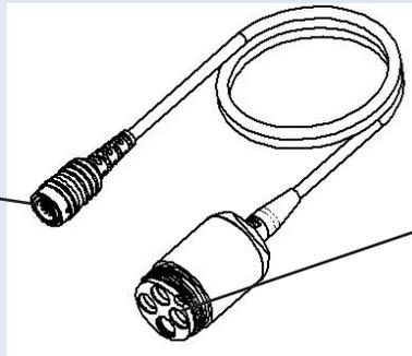
Four ports for user-replaceable sensors. Ports accept a temperature/conductivity combo sensor, DO sensor, and any combination of two ISE sensors among pH, ORP, ammonium, chloride, or nitrate. If a port isn't used simply put a port plug in it's place.
