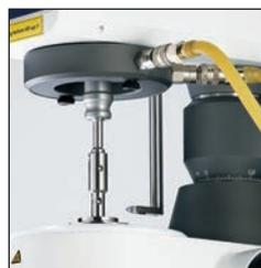
*The optional KE cooling device is required to cool viscometer bearings when testing with temperatures above 70°C.*
