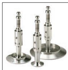
*Choice of cone spindles and plate spindles accommodates all sample types. Plate spindles are used for highly-filled or very viscous samples.*
