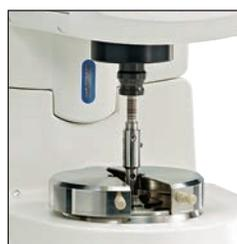
*Thermal Barrier reduces the effects of heat transfer to the environment. Two part chamber provides thermal isolation of the measurement zone.*
