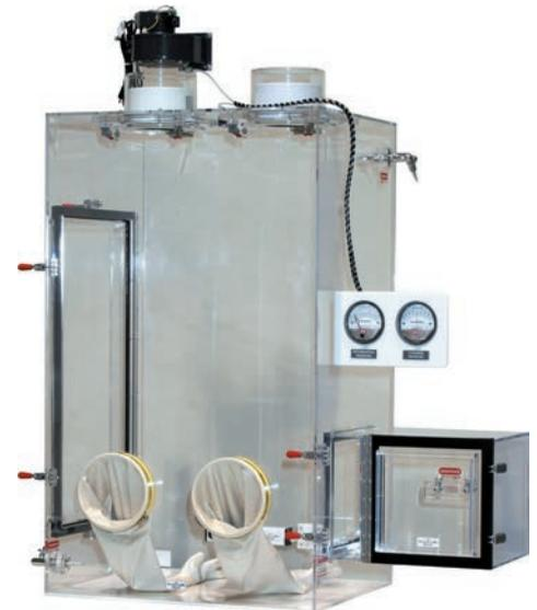
Containment glove box with double HEPA filtration package.
