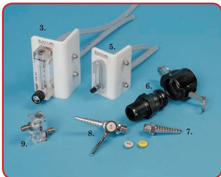
5. **#800-FLOW/D. SMALL FLOW METER** used for smaller chambers and desiccators. Helps regulate gas flow at lower incoming pressures. Kit includes flowmeter, mounting bracket, hoses and ring clips. Range "5-50 SCFH."
