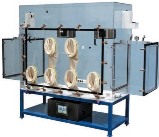
Temperature & Humidity controlled glove box for analysis material.
