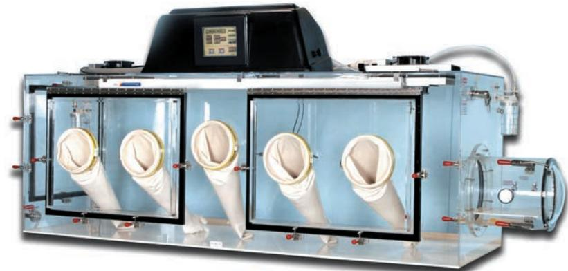
Fitzmill glove box with temperature and humidity control.
