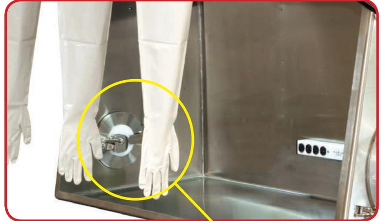
The RTP, “Rapid Transfer Port” provides containment during material transfer. For use with stainless steel transfer canister.
