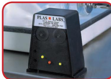
**800-AS/SPI, Anti-Static Ionizer.** Emits alternating positive and negative ions, removing static inside the glove box. This is a non-air assisted static eliminator, (no blower / no fan). The 800-AS/SPI is perfect for working with fine powders and chemicals.
