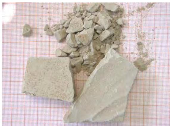
**Fig. 3:** Mud sediment sample before and after manual pre-crushing with a hammer
