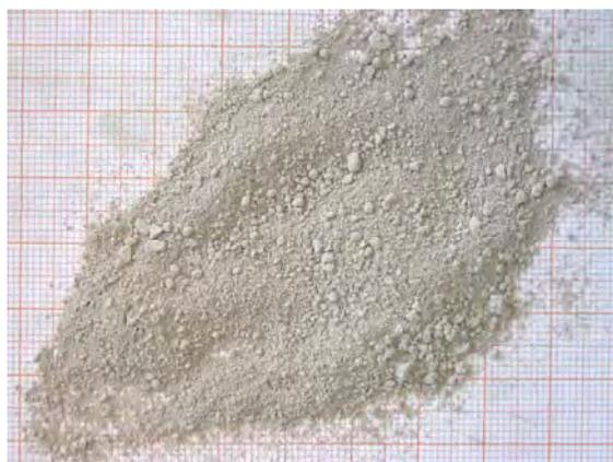
**Fig. 4:** Mud sediment sample after grinding in PM 100 for 5 min.
