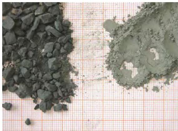
**Fig. 1:** Cement clinker sample before and after grinding in PM 100 for 5 min.
