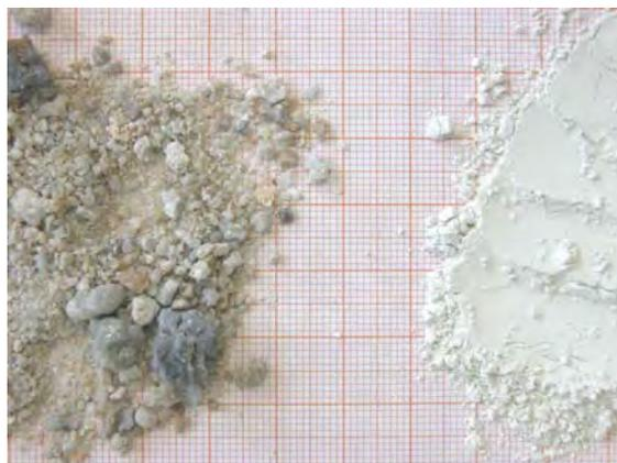
**Fig. 2:** Slag sample before and after grinding in PM 100 for 5 min.
