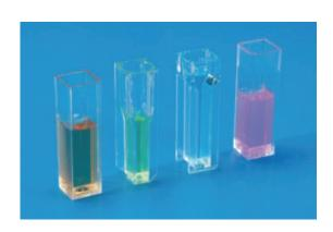
Disposable cuvettes for spectroscopy, in optical-quality PS and UV grade PMMA with optical windows for optimum transmittance when using wavelengths from 340 nm to 800 nm (PS) and from 280 nm to 800 nm (PMMA). The range  $\pm 1\%$  absorption, this is the vital when batch analysis is being undertaken.
