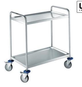
Made of CNS 18/10, material no. 1.4301. All shelves are produced with an all-around raised profile edge. This prevents anything from slipping over the edge. The load capacity per shelf is 80 kg. Wall bumpers made of plastic (polyamide) on all four corners protect against damage.
