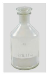
For the determination of dissolved oxygen in water. The measured capacity is specified to  $\pm 0.01$  ml. With a white labelling area. Each bottle and its stopper is marked with a unique, matching identification number.
