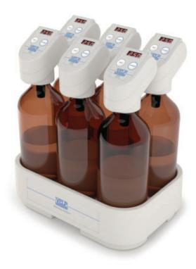
Measuring systems for the reliable determination of 90 to 999 ppm BOD. Complete with sensor heads and multi-position magnetic stirrer.
